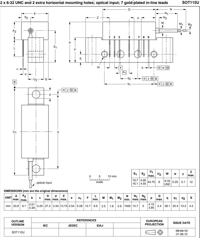
Rectangular single-ended package; aluminium flange; 2 vertical mounting holes; 2 x 6-32 UNC and 2 extra horizontal mounting holes; optical input; 7 gold-plated in-line leads
